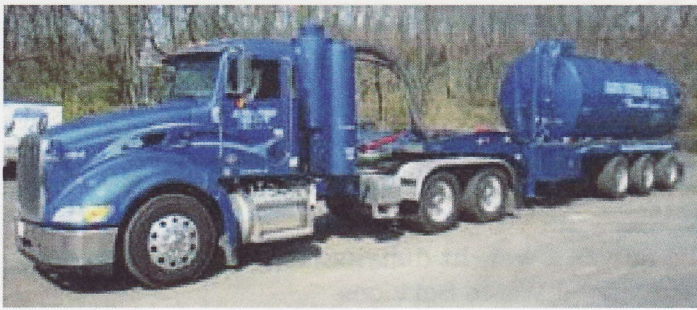
The VacSimizer unit shown with wheels tucked under the tank for maneuverability on the job site.
