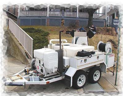
It is a small high pressure hose with a special tip that direct a high pressure stream of water forward to cut the blockage in the pipe and 3 smaller jets of water shooting backwards from the tip to propel the tip forward while moving the debris back.
