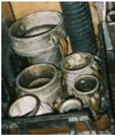
2. **Fittings** – These are usually aluminum or some times stainless steel adapters used for hooking *hoses* to *tanks* or other *hoses*. There are male to male, female to female, size converters for 3” to 2”, 4” to 3” and 6” to 4”. We also have male and female end caps for the *hoses* and *valves*.
