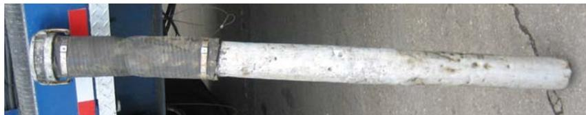
and 4 or 5 feet long with a *fitting* on one end. It is used to more easily pump out below ground *tanks* or *catch basins*.
