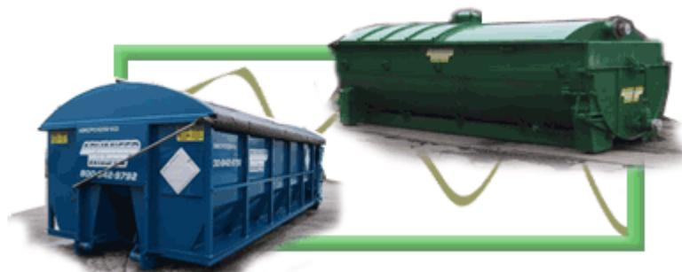
16. **Vacuum box** (Above Green) – This is a *bulk* container used for liquid material. They have a capacity of 5000 gallons but rarely move that much because of weight restrictions. They are picked up and delivered with a *roll off trailer* and filled with the aid of a *super sucker* or *hi-vac* truck. The liner for a *vacuum box* is called a bladder bag.
