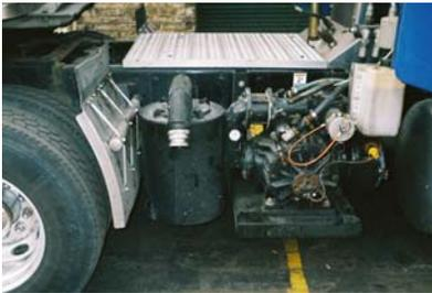
9. **Vacuum Pump** – This is the unit that creates the vacuum (suction) or pressure in the *tanker*.
