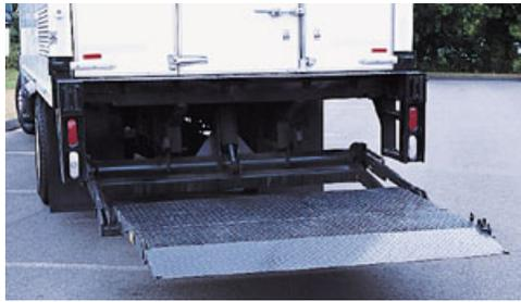
21. **Lift Gate** – This is mounted to the rear of the *van trailers* and *van bodied straight truck*. This allows us to lift *drums* from ground level into the trailer or truck.
