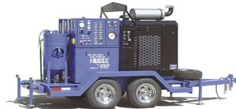
20. **Jetter** – This is a unit designed for cleaning out pipe, such as an underground sewer line.
