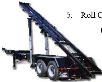
5. Roll Off Trailer – This is a frame trailer used for picking up, transporting and delivering *roll off boxes* and *vacuum boxes*.
